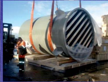
To reduce noise during free venting of steam or gas (safety relief valve), **blow off silencers**, preferably with expansion stages (orifice) will be installed. At the expansion orifice the media is streaming through several cylindrical stages and will be expanded more silent. For further sound reduction the noise will be absorbed
