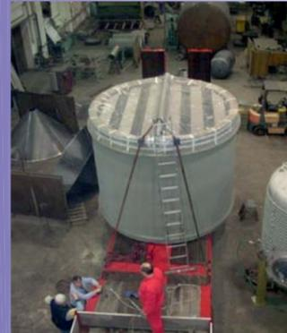
In cases where noise emitted from exhaust ducts or openings (Gasturbines, compressors, etc.) must be reduced effectively absorbing silencer splitters (baffles) are used. We are specialised in:
